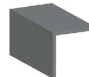
FEA38x38x1.59 38.1mm x 38.1mm x 1.59mm Lengths (mm): 3100 ALL FINISHES AVAILABLE
